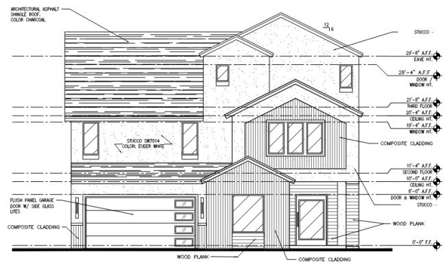
FRONT ELEVATION - CONTEMPORARY 3 STORY
