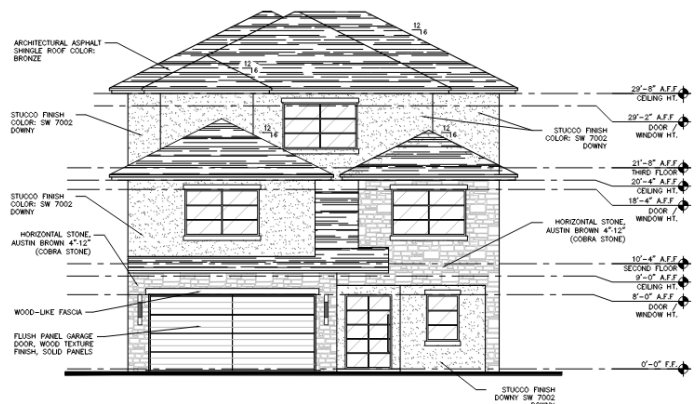
FRONT ELEVATION - TRANSITIONAL 3 STORY
