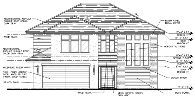
FRONT ELEVATION - TRANSITIONAL 2 STORY
