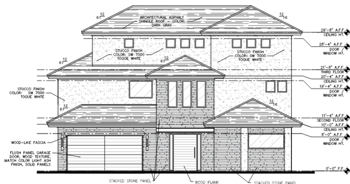
FRONT ELEVATION - TRANSITIONAL 3 STORY
