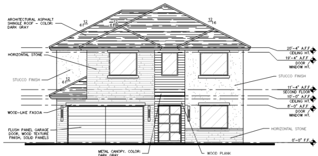
FRONT ELEVATION - TRANSITIONAL 2 STORY
